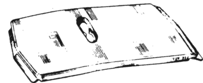
74-3964 Replaces: 96447459 CLIP-MOULDING FRONT DOOR (LOW CENTER) REAR DOOR (LOWER FRONT) Chevrolet, Olds, Pontiac '73 UNIT PACKAGE 50
